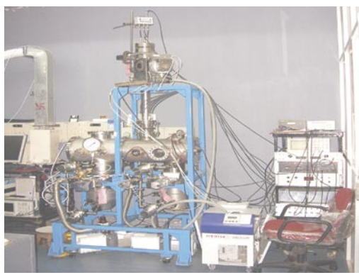
Fig.5. Photograph of the integrated system of MB-TOF-REMPI setup.
