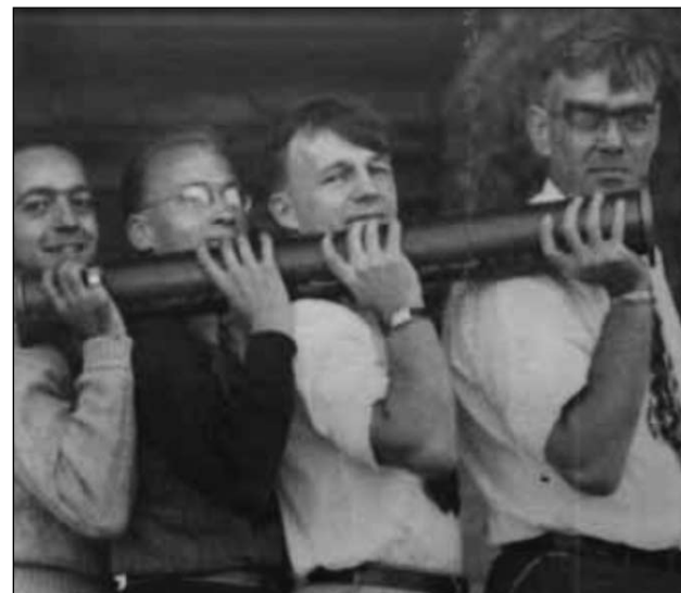
Fig 3: A section of the first linear electron accelerator, which operated at Stanford University in 1947. Eventually 3.6 m long, it could accelerate electrons to an energy of 6 MeV. (Courtesy Stanford University)
