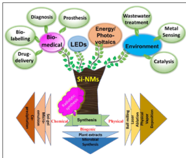
Figure 3. Schematic representation of major physical, chemical, and biogenic methodologies for synthesizing Si NMs and their applications across diverse fields.
